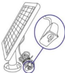
Insert the micro-USB plug into the micro-USB port on the camera. Ensure area is sealed with white weather proof rubber bung (Optional Accessory).
